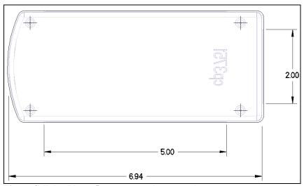
Figure Cellular Phone 5 Bottom Drawing, Top View
